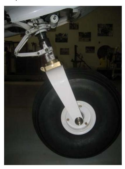
In this configuration the nose strut tube does not require cutting. The nose fork and integrated block are removed and new block is attached to strut tube using the existing holes. The new block and nose fork are installed in accordance with instructions provided.
