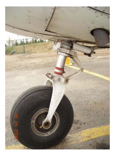
In this configuration the nose strut tube does not require cutting. The nose fork and integrated block/steering collar are removed and new block is attached to strut tube using the existing holes. The new block and nose fork are installed in accordance with instructions provided.
