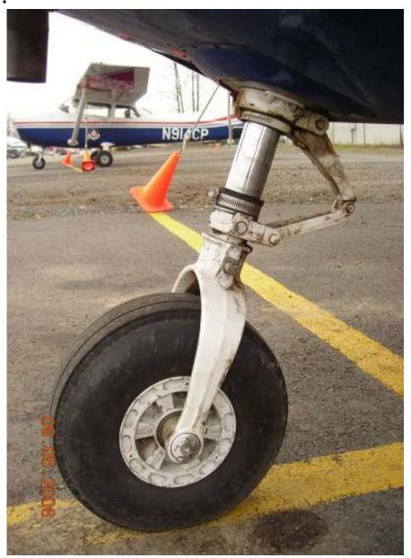
In this configuration the nose strut tube needs to be cut off. This was an <u>improper</u> installation made by a customer. The new block should be installed in place of preexisting block/steering collar. Strut tube is cut off flush with bottom of fork. The torque link attaches to new Airglas block. The new block and nose fork are installed in accordance with instructions provided.
