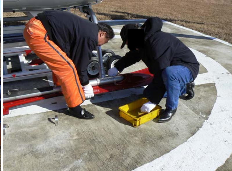
Position ski to insure the skid is tight against the socket face.
