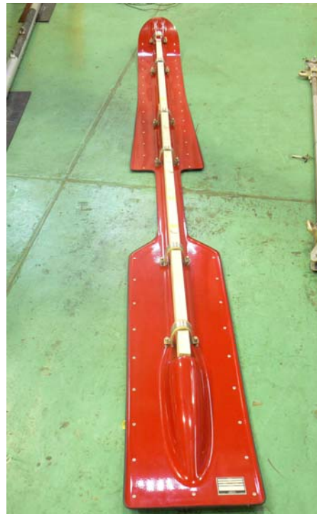
Ski with 2x3 stiffener still attached after packaging has been removed.
