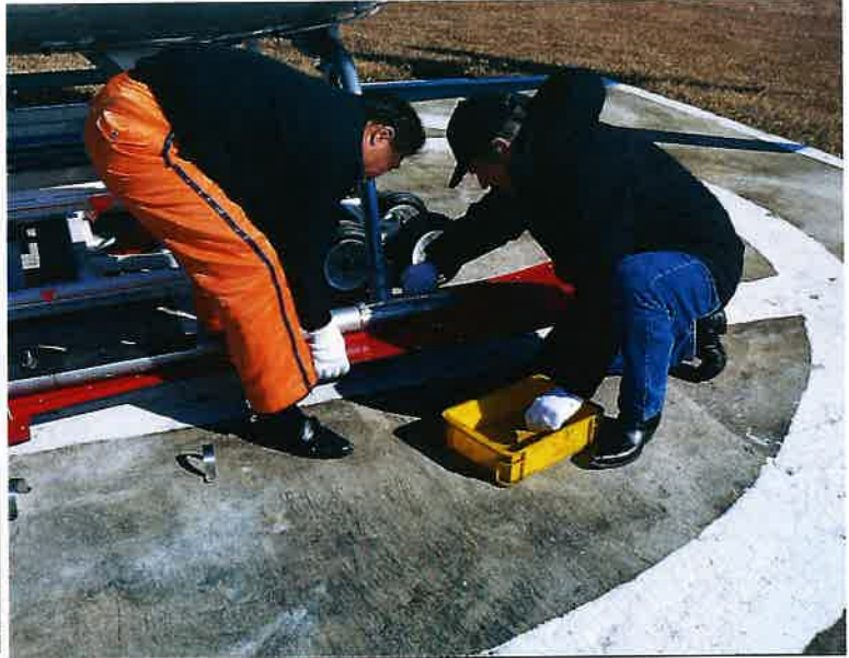
Position ski to insure the skid is tight against the socket face.
