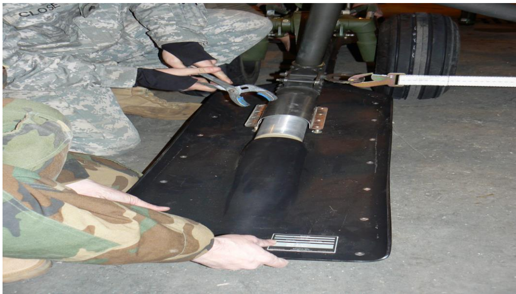
(L2700-OH58D-6 Adapter installed onto skid)
