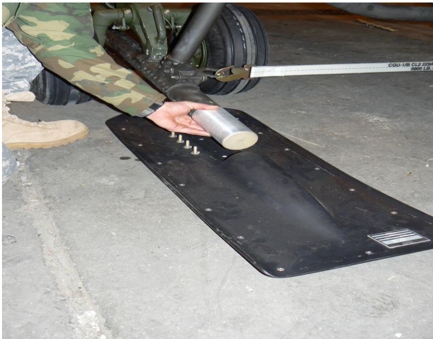
(Adapter installed onto skid tube)
