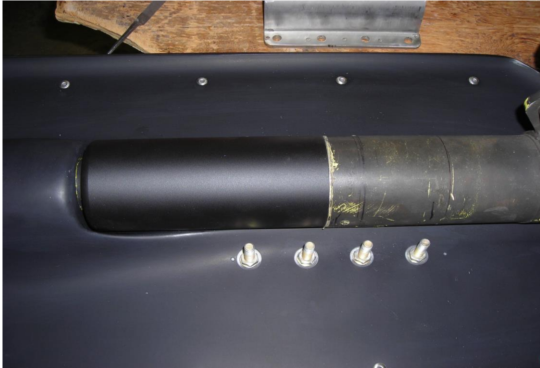
(L2700-OH58D-6 Adapter installed onto skid)
