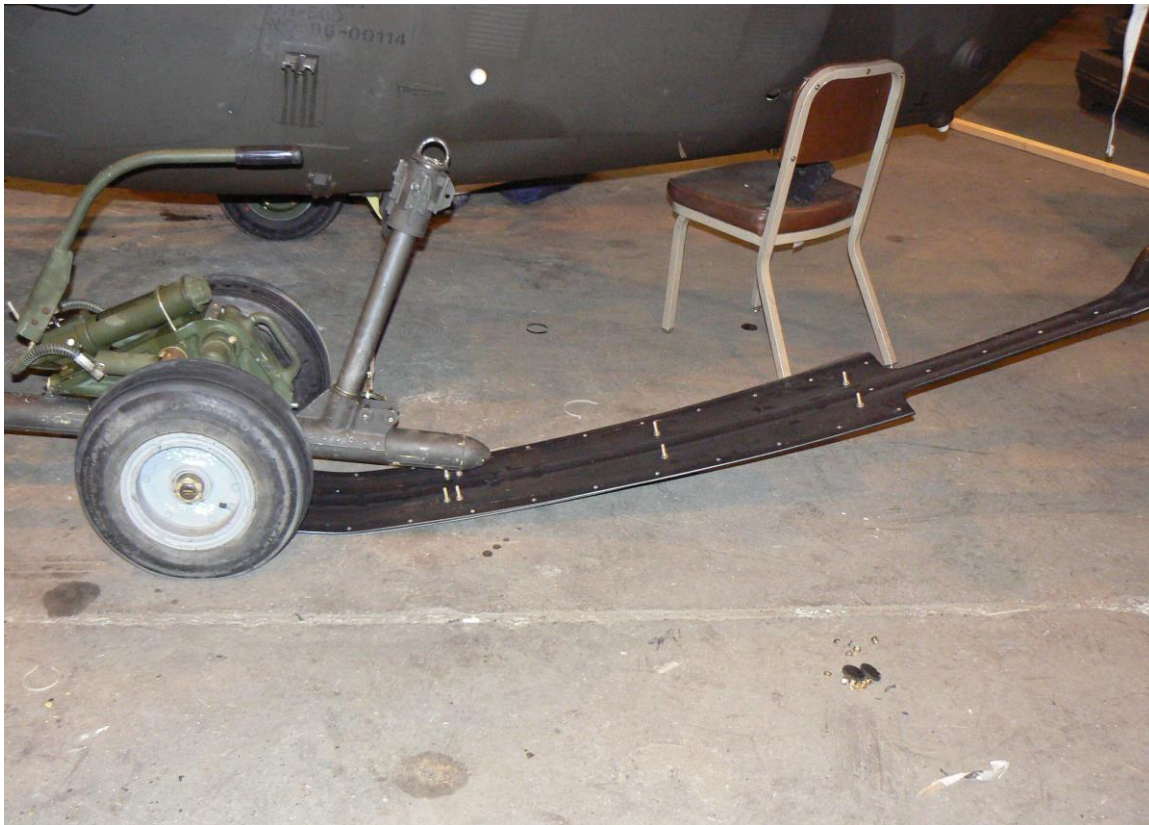
(Ski tail lifted up for installation)
