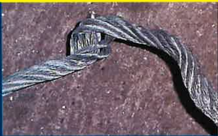
KINKED/ WORN CABLES
