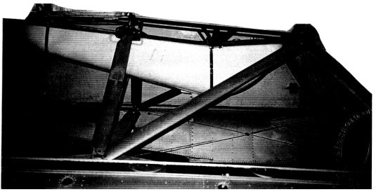
LTC18 Fuel/Cargo pod installed, view from right side (LC18 similar). Current production doors are on right hand side.
