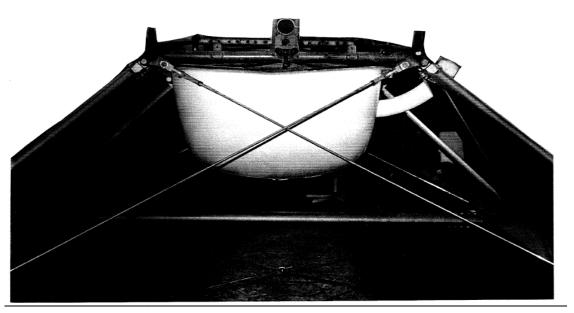
LTC18 Fuel/Cargo pod installed, view looking aft (LC18 similar).
