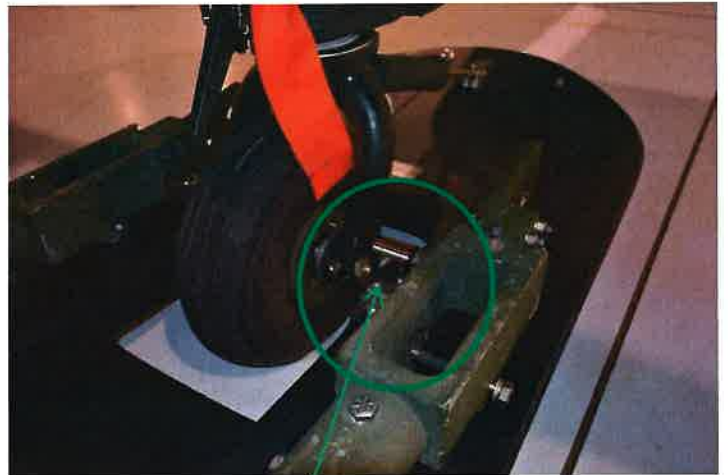
Tail ski with L20500A-14-2 Tow Bar Adapters reinstalled and connected to tow bar.
