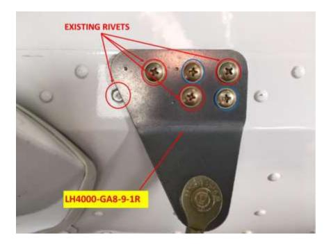
7. Remove the aircraft interior floor inspection panels between FS. 87 and FS. 170. Refer to drawing LH4000-GA8 sheet 2 detail B. Locate the LH4000GA8-9-2L as shown in detail B on the left hand side of the aircraft. Note the rivets that the bracket will cover. Drill out the two existing rivets using a #30 drill bit. Enlarge the forward rivet hole using a #9 drill bit. The top edge of the LH40009GA8-9-2L and the packer part #LH4000GA8-9-1P must be ground to fit
