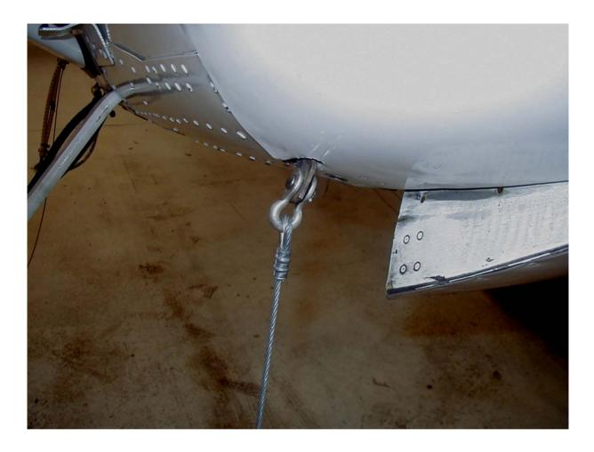
Note: Lower cowl will need to be notched to allow for bracket installation.
