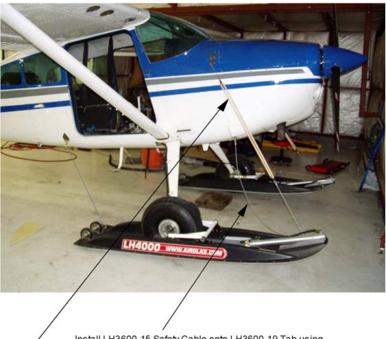
Install LH3600-15 Safety Cable onto LH3600-19 Tab using AN395-19 Clevis pin and AN380-3-2 Cotter pin
